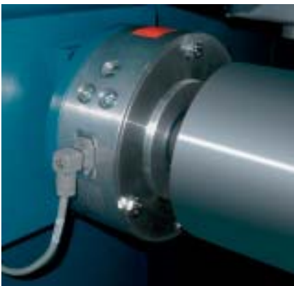
Flange load cell PD 25 at infeed into sizing bath
