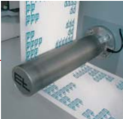
Sensor roller PD 40 on re-rolling machine
