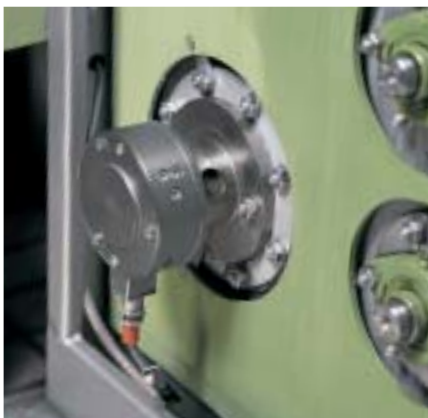
Flange load cell PD 23 on washing machine
