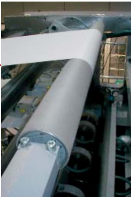
Sensor roller PD 30 on rotary offset press
