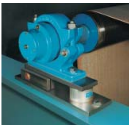
Block load cell PD 7 on paper machine
